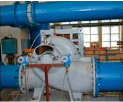
Double suction pump testing
