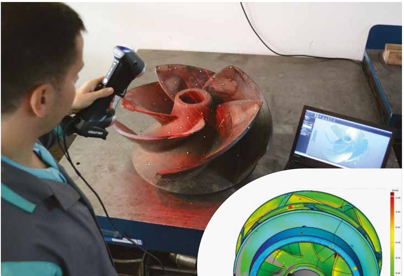
Carrying out a laser scan of a cooling water pump impeller
